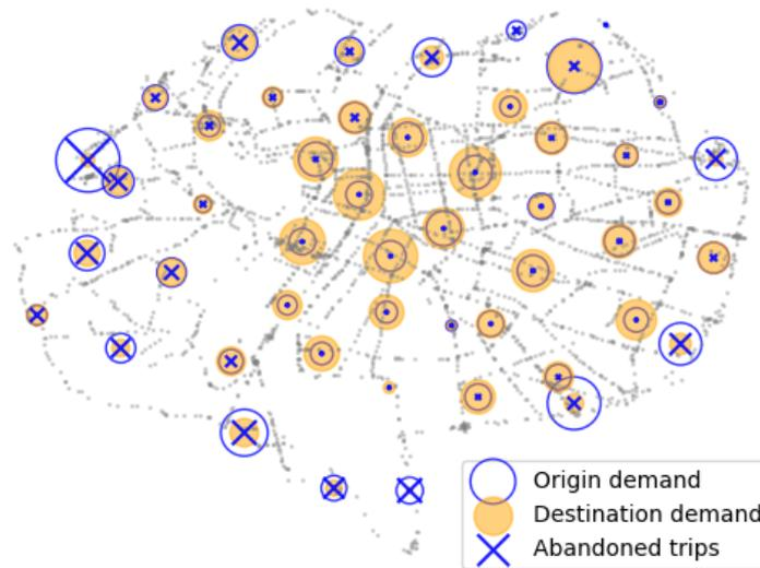
Figure 16: Demand and loss aggregated at the centroids of 50 zones from pool scenario of Method 3
